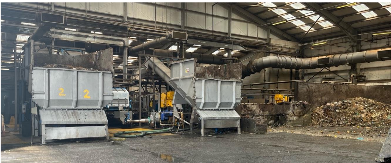
Figure 5-3: Biogen Bygrave feedstock receival shed, including unloading areas, blending systems and air extraction system, UK, June 2024
