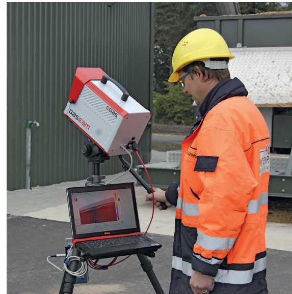
Gas leak detection during the maintenance
