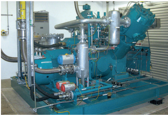
Compressor Package TVZ 900-200 Ex for e.g. grid injection
