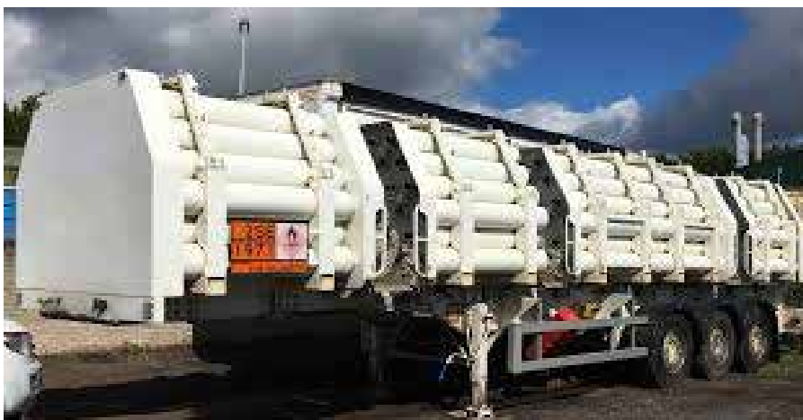
Steel Tube Trailer
