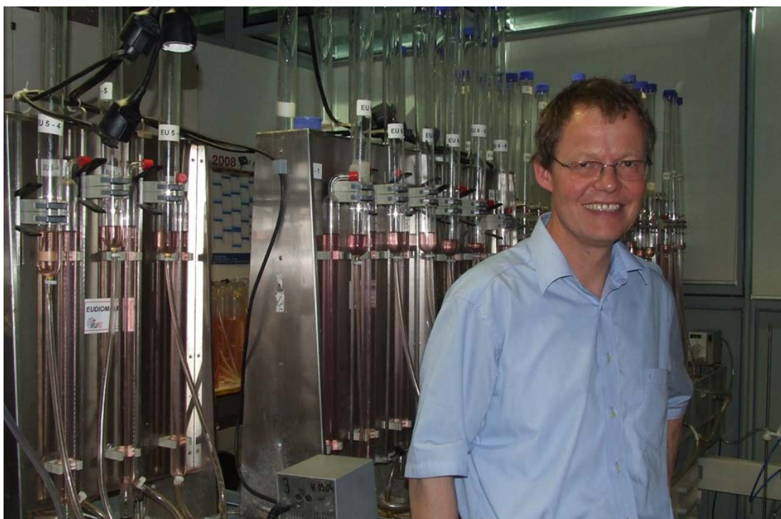
Figure 2: Prof Thomas Amon in front of the experimental setup, what is measuring the actual production of methane in crops at BOKU (Vienna).
