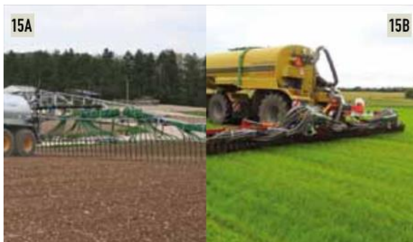
Figure 4: Left – dribble bar application of biofertiliser. Right - direct injection of biofertiliser (Seadi et al., 2010) .
