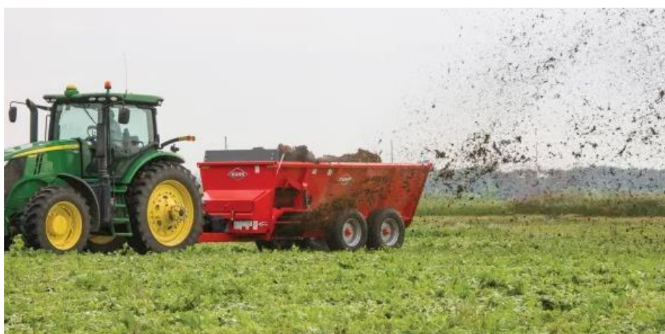
Figure 5: Typical manure spreader, also suitable for spreading solid biofertiliser (Source: Kuhn.com).
